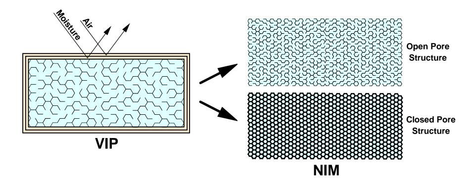
NIM - A basically homogeneous material with a closed or open small nano pore structure preferably with an overall thermal conductivity of less than 4 mW/(mK) in the pristine condition.
